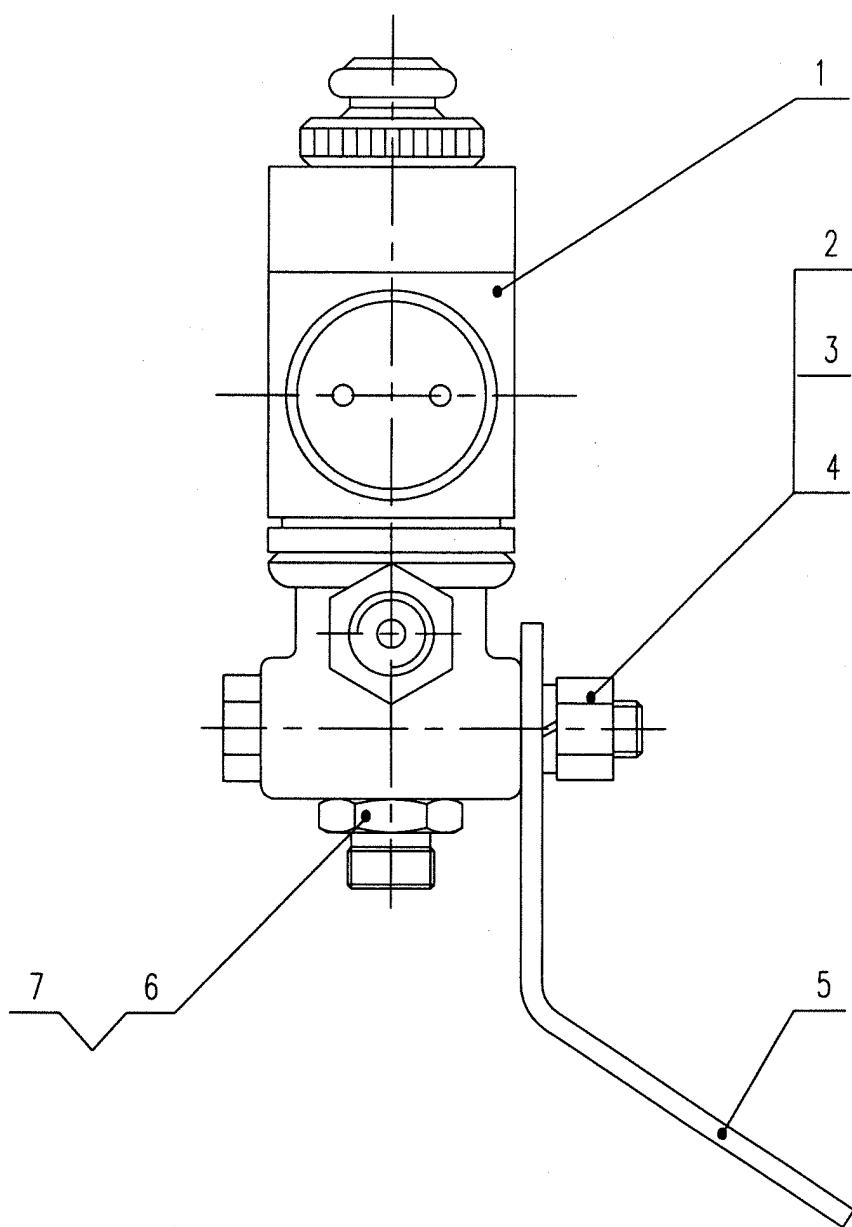
XZ16K.41.5A 差速电磁阀安装 Solenoid Valve Assembly
