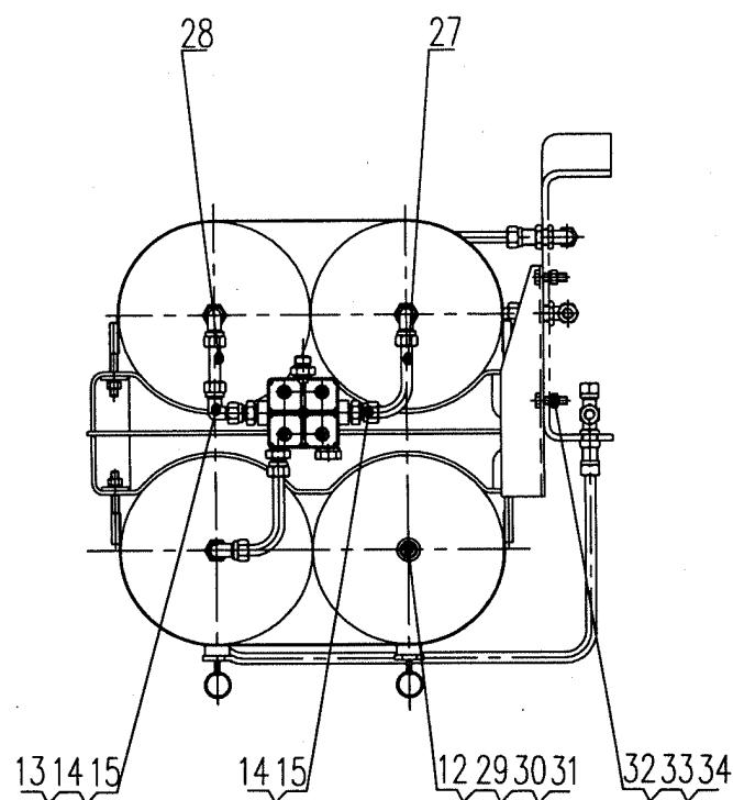
XZ16K.39A 贮气筒安装 Air Reservoir Assembly
