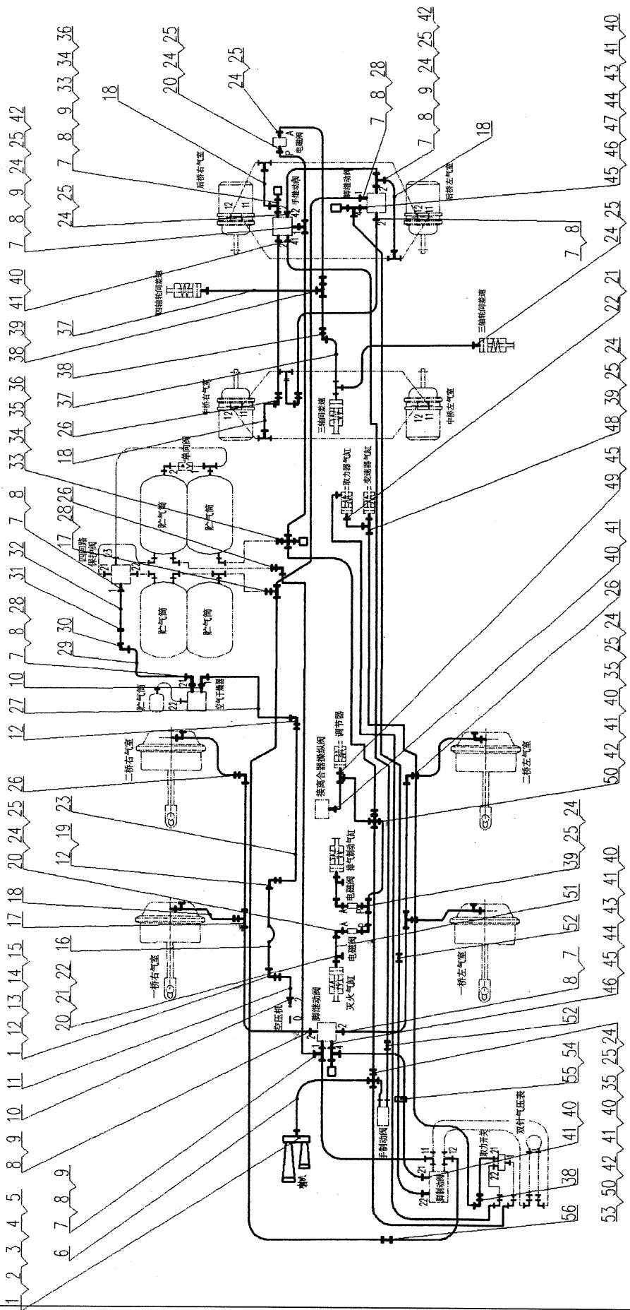
XZ16K.42A 气路布管图 Air Circuit Pipe Assembly
