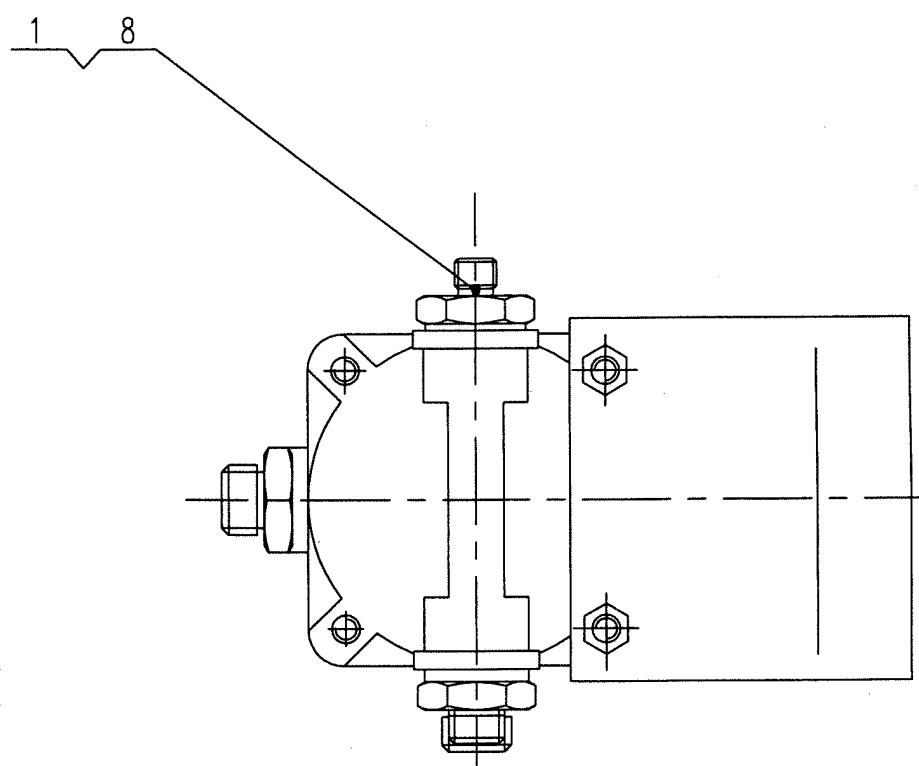
XZ16K.41.4A 手继动阀安装 Hand Relay Valve Assembly
