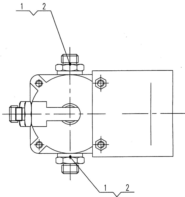
XZ16K.41.3A 脚继动阀安装 Foot Relay Valve Assembly
