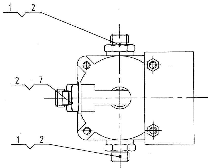
XZ16K. 41. 1A 脚继动阀安装 Foot Relay Valve Assembly
